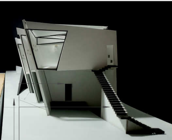
House has two entrances/exits Staircase in the back is penrose that reaches from basement to the second level Slope lets natural light to reach the basement
